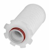
**mdi** AseptiSure® KR Cartridge filters incorporate a low protein binding PES membrane with polypropylene drainage layers to ensure pH compatibility from 1-14 making these ideal foralkaline fluid streams.
